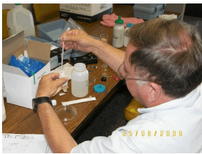
Figure 9. Coliform bacteria test on river water.
