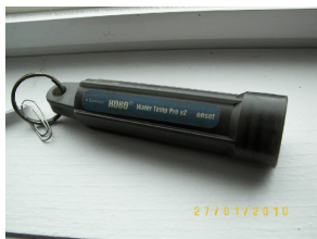
Figure 5. HOBO V2 temperature logger.
